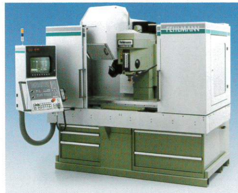
1994: PICOMAX 82 HSC the HSC era, with 30,000 rpm
