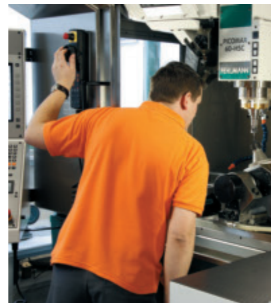
Important feature of the FEHLMANN PICOMAX 60-HSC is the good accessibility to the machining area and the fact that a vice and a dividing & swiveling nit as 4th and 5th axis can simultaneously be installed on.
